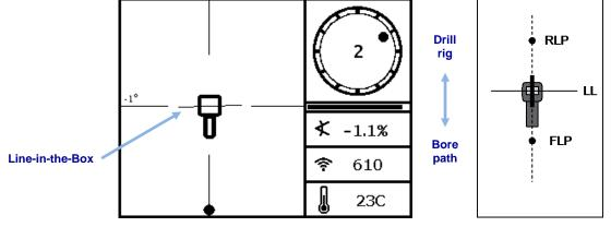
8. Position the receiver so the LL aligns with the horizontal crosshair.
