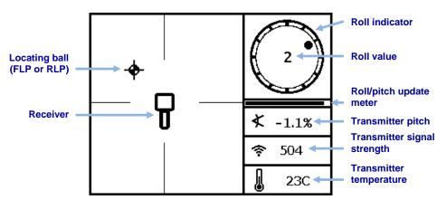
Typical Locate Screen with Transmitter in Range
