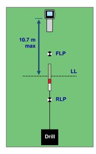
Positioning the Receiver for Target Steering
