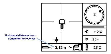
**Target Steering Data on the Receiver**
