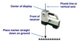
**Plumb Line for Marking Locate Points**
